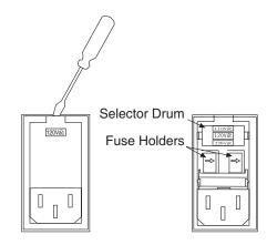
Figure 39. Power Input Module
